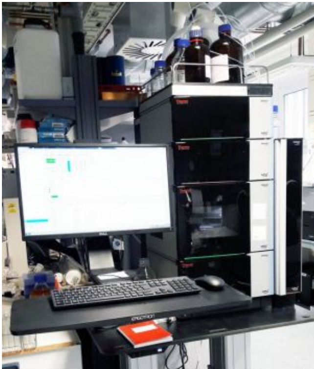
Thermo Vanquish Horizon UHPLC
