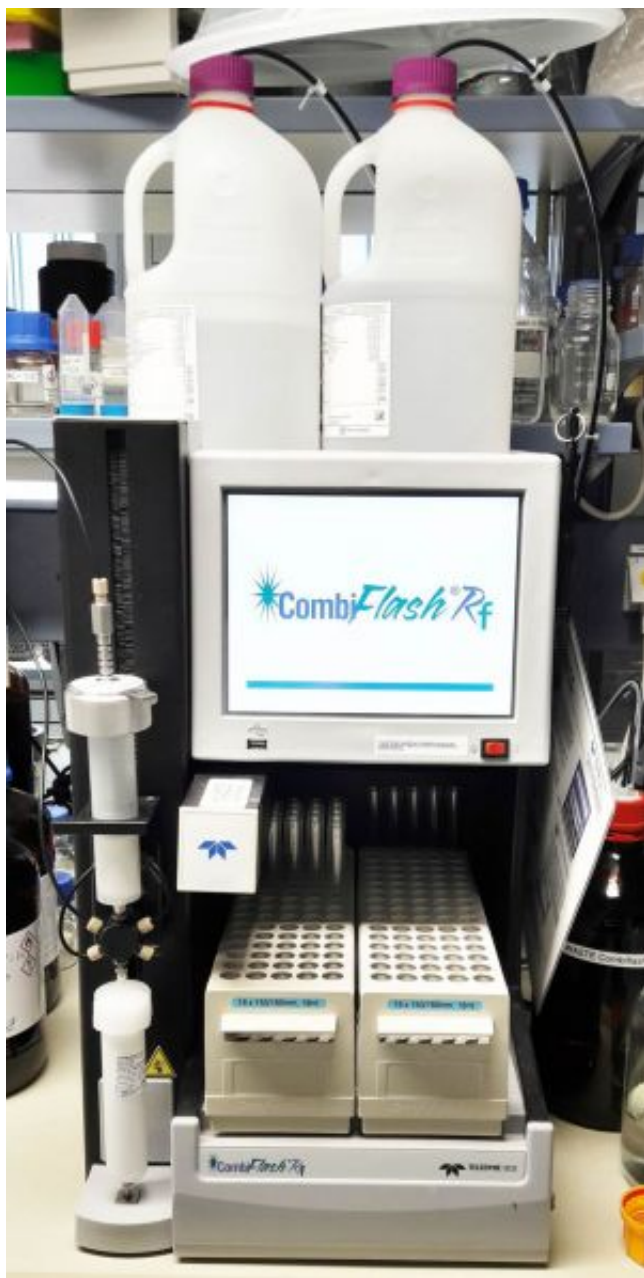
Flash-Chromatography plant Teledyne Isco Combi
