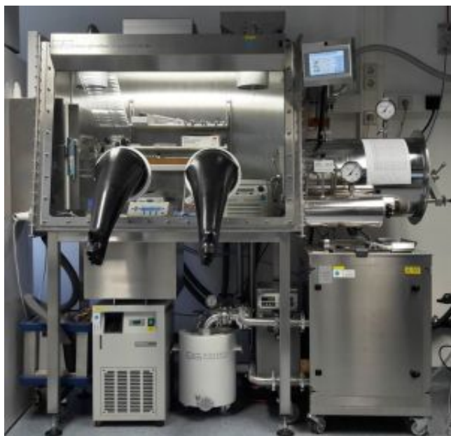
GS Glovebox with freezer and gas cooler for inert tasks
